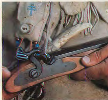
An example of the earlier flintlock rifle and the later-developed percussion cap rifle. Both were loaded from a powder horn, at the muzzle. The flintlock also had to be primed with powder at the breech.
